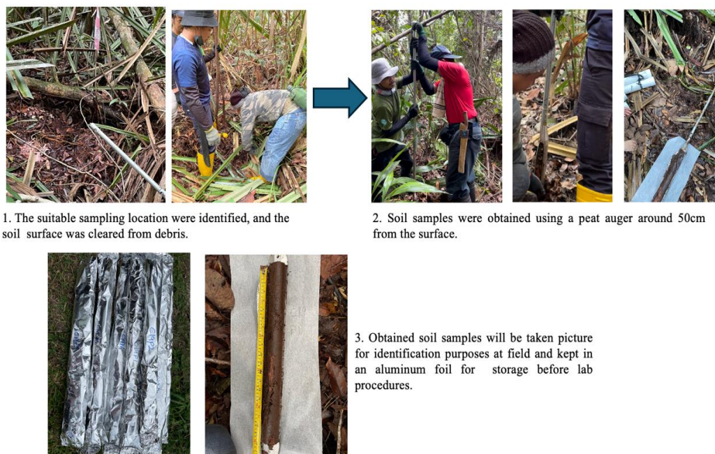
Figure 3. Soil sampling conducted at 50 cm depth in the field and sample storage
